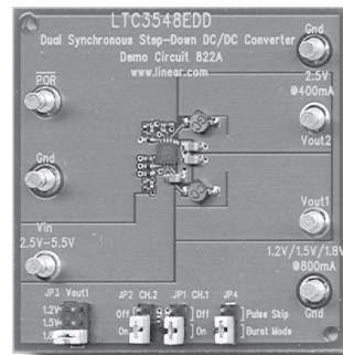
Figure 1. Two DC/DC regulators occupy less than 0.2in 2 of board space
